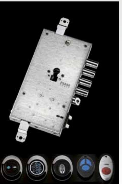
door control panel is also used to customise programming of the lock. For example enabling/disabling the electronic keys, keypad codes, remote controls, etc. The lock is also provided with a safety cylinder operated by normal mechanical keys: if the electronics needs maintenance, the door can be opened and closed like all models equipped with a standard lock.
